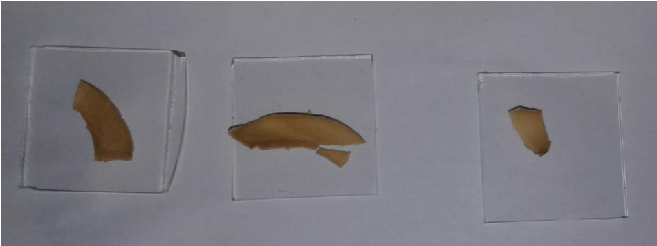
Figure 1. 20 µm geopolymer foil obtained by spin-coating
