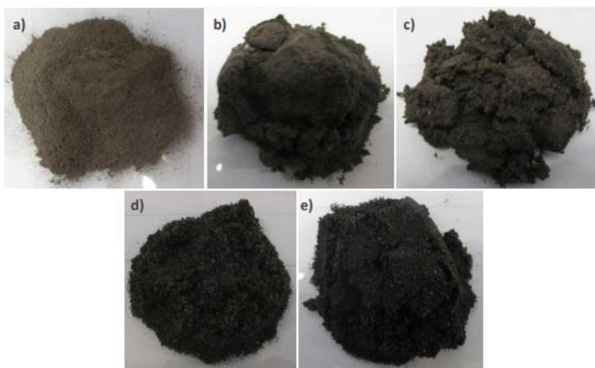
Figure 1. Samples of fly ash from TPP Nikola Tesla a) FA1, b) FA2, c) FA3, d) FA4 and e) FA5
