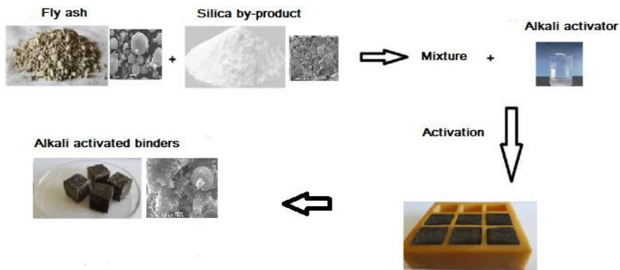
Fig. 1 Process of alkali activation of fly ash
